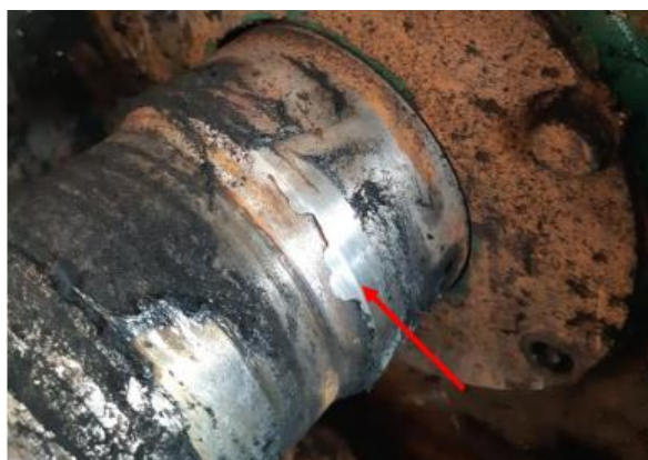
Figure 5 There are traces of hardfacing on the shaft.
