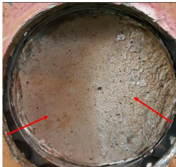
Figure 3 Shaft fracture condition.
