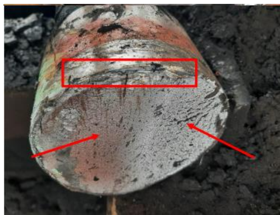
Figure 4 Shaft fracture condition
